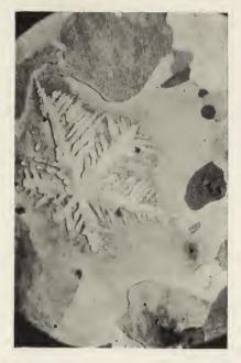
Fig. 9. (x 33 Diameters. Vertical Illumination.) Dendrites of Cadmium. Showing relation to crystallization.
